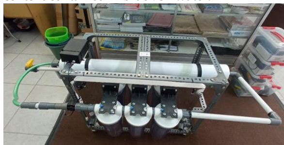
Figure 6 Brackish Water to Raw Water Filtration System
