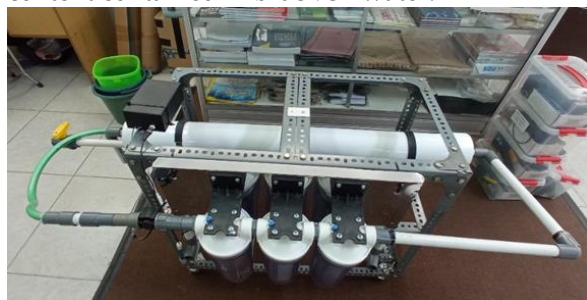
Figure 6 Brackish Water to Raw Water Filtration System
