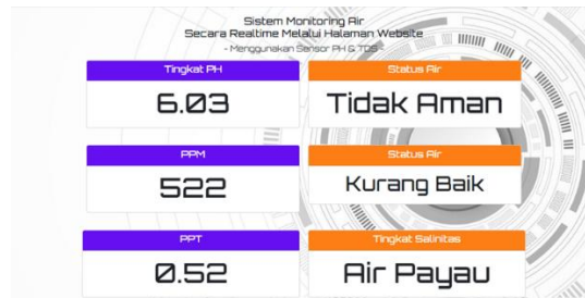
Figure 7 Web-based monitoring view of water conditions
